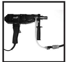
1. Connect the 350mm long water hose (8) on DDM2 - 110 to a suitable water supply by push fitting into a "Gardena" or "Hozelock" type fitting which is attached to a hose pipe. The hose pipe could be typically between 5m - 20m in length.
