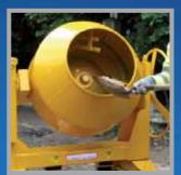
Ridge, reinforced drum to prevent distortion
