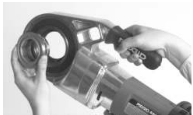
Figure 2 – Installation of 11-R Die Head Adapter
