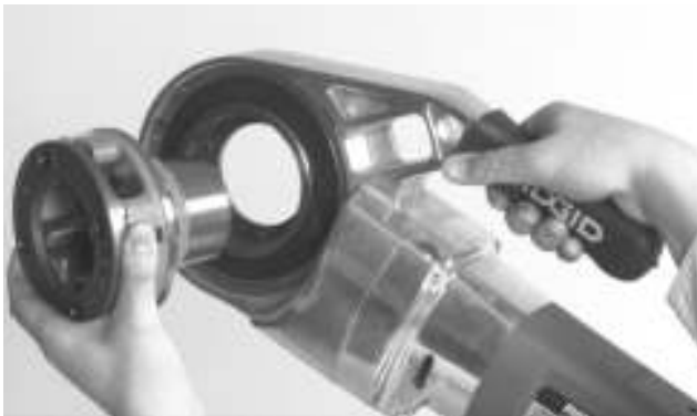
Figure 3 – Installing No. 11-R Die Heads
