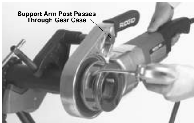
Figure 7 – Threading Pipe and Applying Oil
